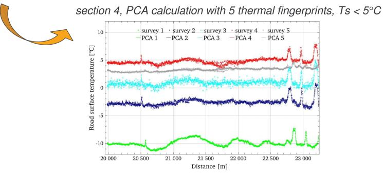
excellent fit between PCA results and local field mesurements
