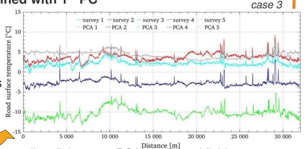
excellent fit between PCA results and field mesurements
