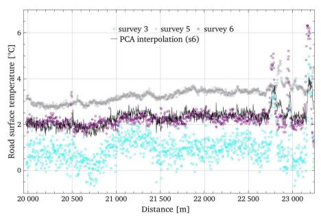
excellent fit between interpoated PCA results and local field mesurements
