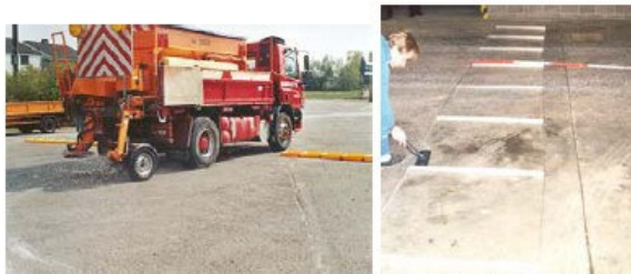
Overview of the initial technical control of spreaders (for wet salt (left) and dry (right) spreading – Walloon region
