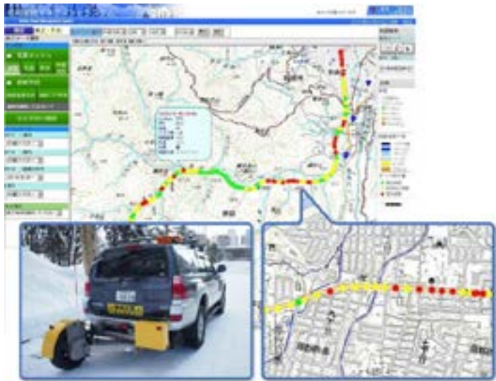
Top: Winter road friction provision system display Left bottom: Test vehicle with a continuous skid-resistance measurement device. Right bottom: Enlarged route map showing measured skid resistance FIGURE 21 - WEBSITE OF WINTER ROAD CONDITION MONITORING DATA
