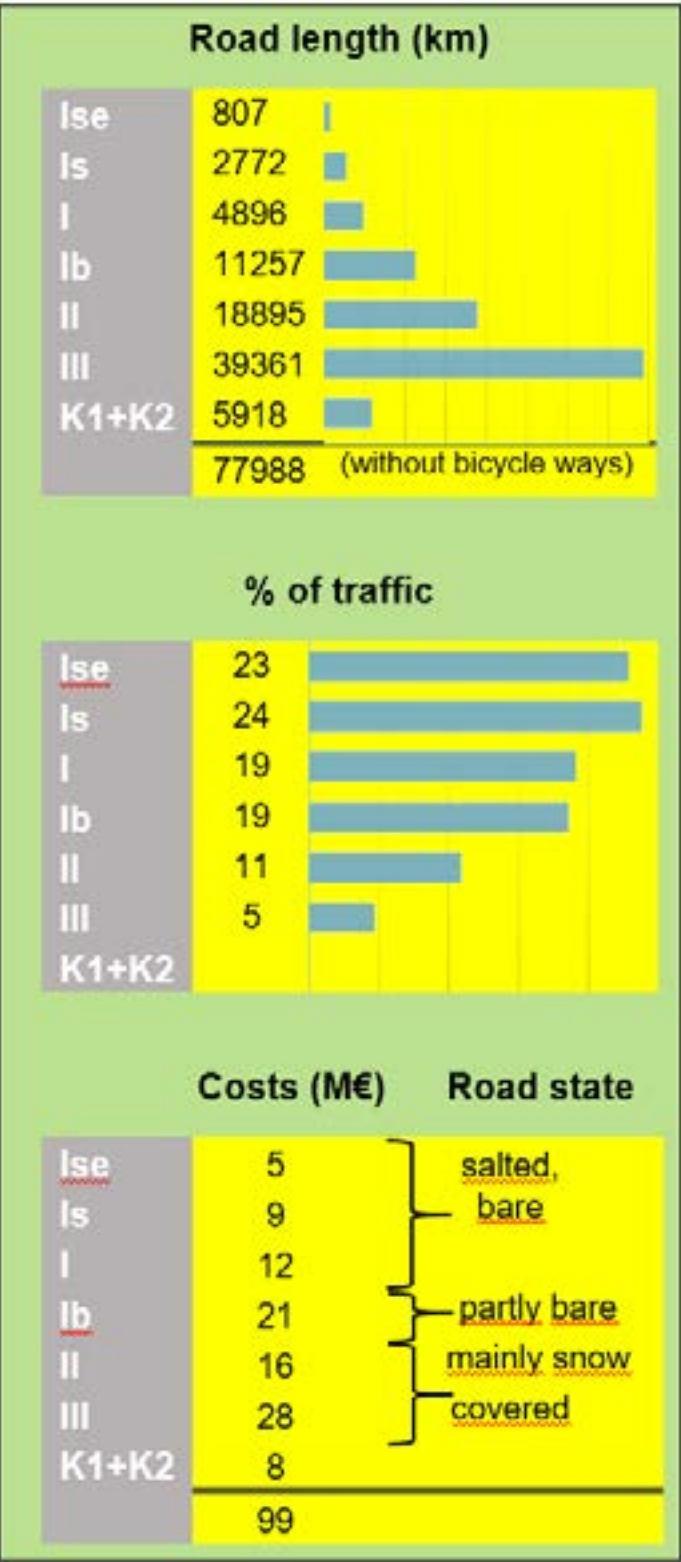
Figure 7 Road lengths, percentage of traffic and costs of winter maintenance in different maintenance classes 2012.
