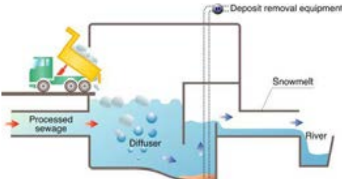
HEAT SOURCE OF SNOW-MELTING TANK: WARM PROCESSED SEWAGE, RESIDUAL HEAT FROM INCINERATION PLANTS, ETC.
