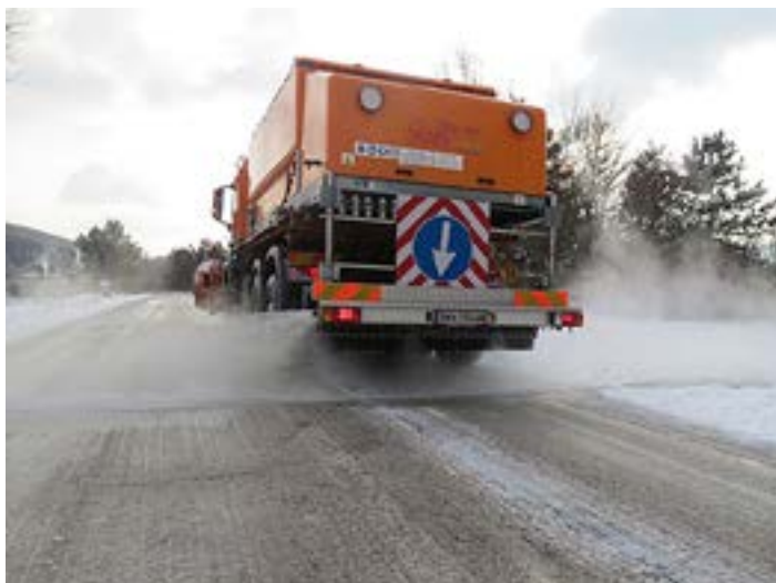
FIGURE 5 – TRUCK "FIRESTORM" WITH BRINE SPRAYING DEVICE
