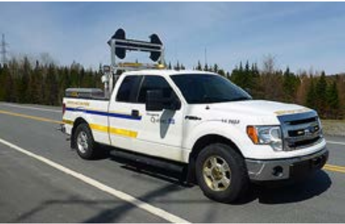
FIGURE 6 – MOBILE ROAD WEATHER STATION
